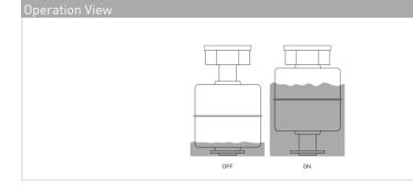
When mounted near ferromagnetic parts switching distance of PLS-045A-3VAI may vary.
